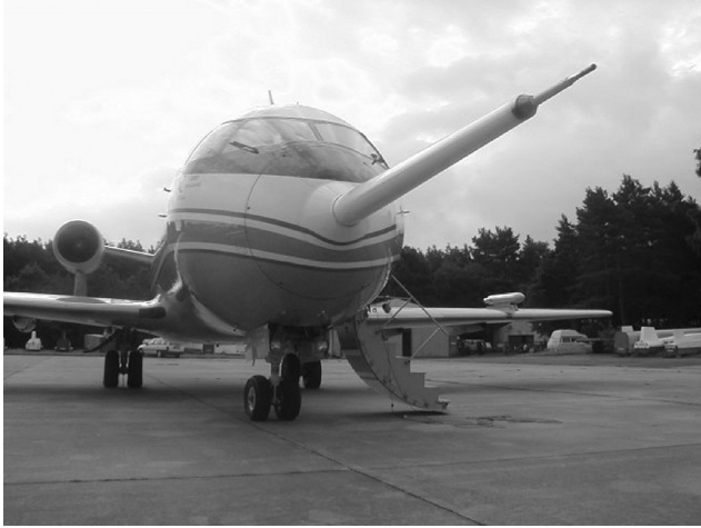
Fig. 1 Test aircraft ATTAS with five-hole probe.
